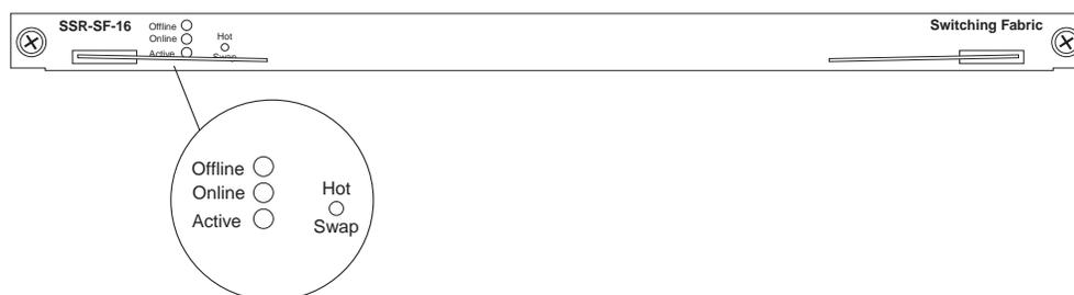
**Figure 8. Front panel of X-Pedition 8600 Switching Fabric module**
